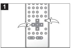
Press the ZOOM button ① once during Normal, Slow or Still playback modes, and the unit will zoom x2. Press once or twice more and the unit will zoom x3/x4. Press yet again to resume normal view. Use the Navigation  $(\blacktriangleleft, \blacktriangleright, \blacktriangle, \blacktriangledown)$  buttons ② to move the image on the TV screen. This is not available on all discs.
